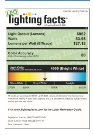
Photometric values based upon tests performed in compliance with LM-79. IES files can be downloaded at www.ilp-inc.com
