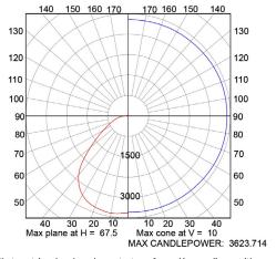
Photometric values based upon tests performed in compliance with LM-79. IES files can be downloaded at www.ilp-inc.com
