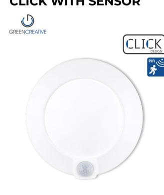
The integral passive infrared sensor of the CLICK surface mount fixture helps deliver a balance between high quality 90 CRI light and energy savings in variable occupancy spaces. Turning on instantly with room occupancy and off after ten minutes of room vacancy, the CLICK provides easy and reliable fixture control and performance.
